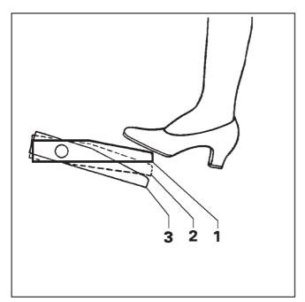
Switch position **1** (inactive) Ironing Switch position **2** Steaming Switch position **3** Lifting the heater plate
