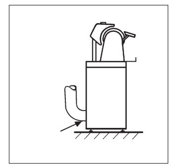
A condensate trap must be installed at the lowest point to prevent condensation from collecting in the duct.
