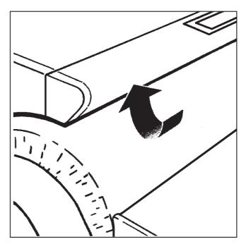
The finger guard is a safety feature to prevent injuries. When the finger guard is lifted, the roller stops and the heater plate raises off the roller.
