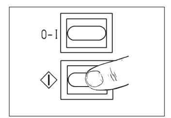
■ Press the <a> "Start" button. The heater plate lowers and the roller turns.</a>
