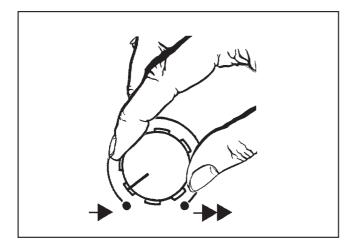
The roller speed can be increased by turning the selector clockwise and decreased by turning it counterclockwise.
